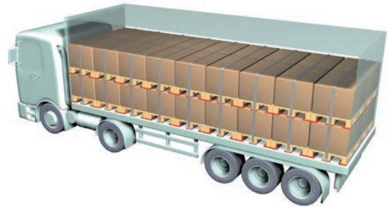
Correct load securing: The anti-slip mats are marked in red here.
